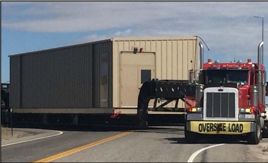
(Above/Right) Turning doesn't seem that difficult until you start to go up! Mark Lemon (900216) maneuvers a Control Building up the mountain turns from Price, UT to Hudson, CO. The total dimensions were 190' long, 16'7" wide, 16'6" high with a gross weight of 254,000 lbs. Mark has been a company driver since 2002.
