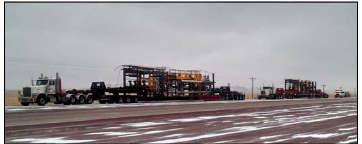
These heater annex skids loaded in Big Cabin, Oklahoma in February and delivered to Alberta, Canada by Wayne Driver (7401) and Darren Jackson (7402) . Dimensions were 170' L x 16'4" W x 16'6" H and 215,000 gross weight.
