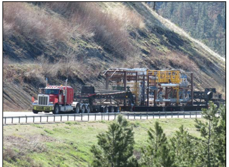
Mark Lemon (900216) hauled this skid module from Big Cabin, OK to Estevan, Saskatchewan, Canada in May. Dimensions were 16' W x 16'6" H and 187' long.
