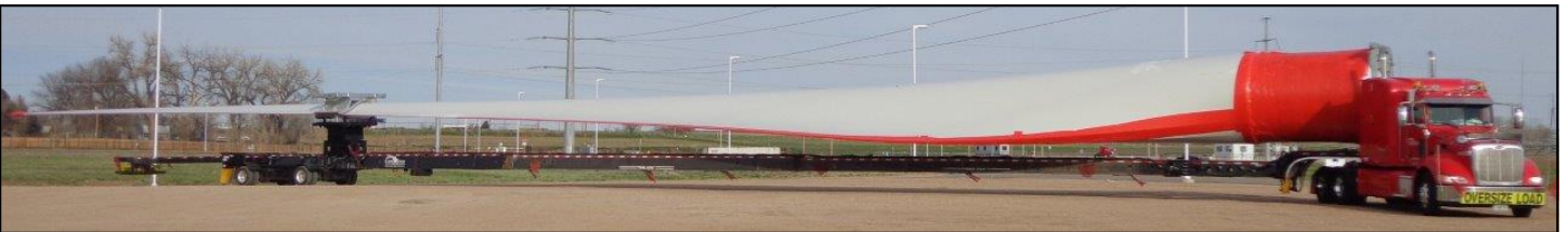
Mike Ptak (900327) loaded and hauled this 57M Vestas blade in Brighton, Colorado in May 2013, with Supervisors Mike Hall and Jimmy Peeler . Load dimensions were 212'6" L x 13' W x 14'2" H. This load had a 29'6" rear overhang.
