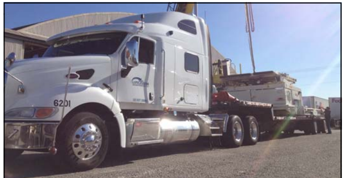
Brian Speakman (6201) hauled this 37,000 pound Commander 15, which is used by Fed-Ex to load freight onto aircraft, to the Burbank Airport.
