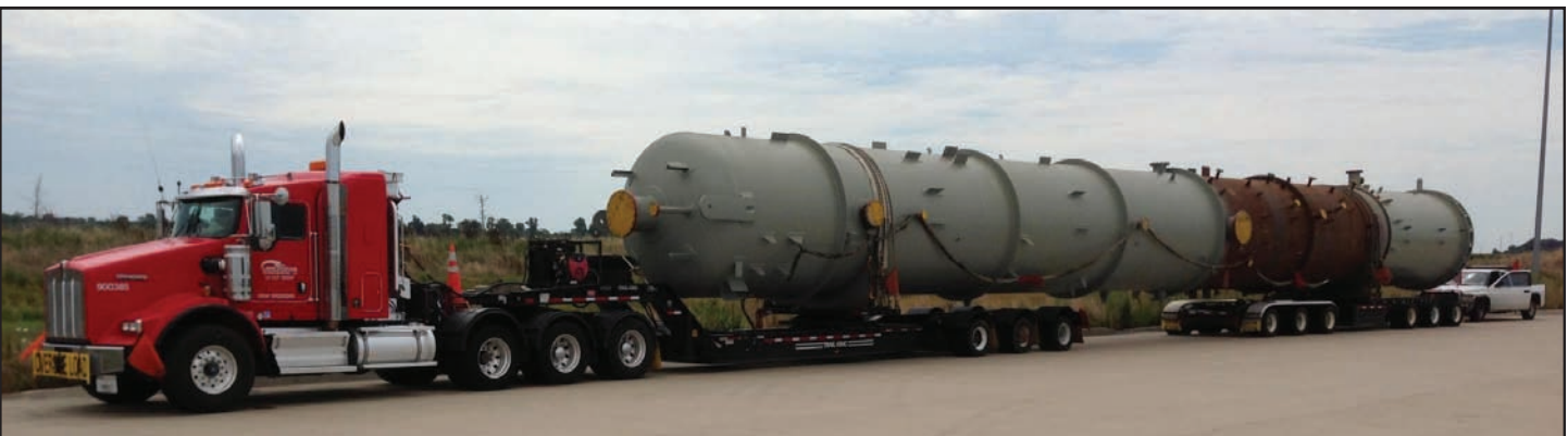
Glenn Kenkel (900385) hauled this regenerator on 13 axles from Longview, Texas, to Morris, Illinois, for Dave Campbell—Kilgore agent. Loaded dimensions were 142' x 11'9" x 15'6" and it weighed 248,000 pounds. Glenn has worked for Lone Star since February 2012.
