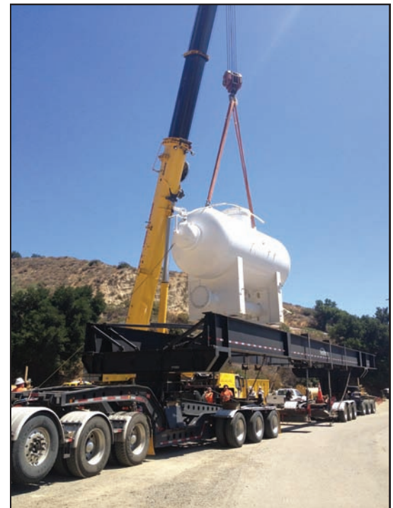
Glenn Kenkel (900385) hauled this regenerator on 13 axles from Longview, Texas, to Morris, Illinois, for Dave Campbell—Kilgore agent. Loaded dimensions were 142' x 11'9" x 15'6" and it weighed 248,000 pounds. Glenn has worked for Lone Star since February 2012.
