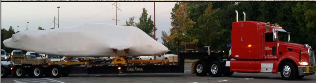
(Below) TL Phillips (8294) , shown with other Lone Star and Shell drivers and escorts, in front of one of three riser joints moved for Shell from Spring, TX, to New Iberia, LA. The loaded dimensions were 200' long, 10' wide, and 14'6" high, weighing 231,000 pounds. TL has been with Lone Star since January 5, 1995.
