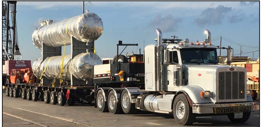
Port of Houston, TX to Baytown, TX continued... (Above) Dennis Rasberry (200112) hauled a third piece, an E413 A/B Exchanger. His load dimensions were 36' long, 6' wide, 14' 6" high, weighing in at 113,000 pounds.
