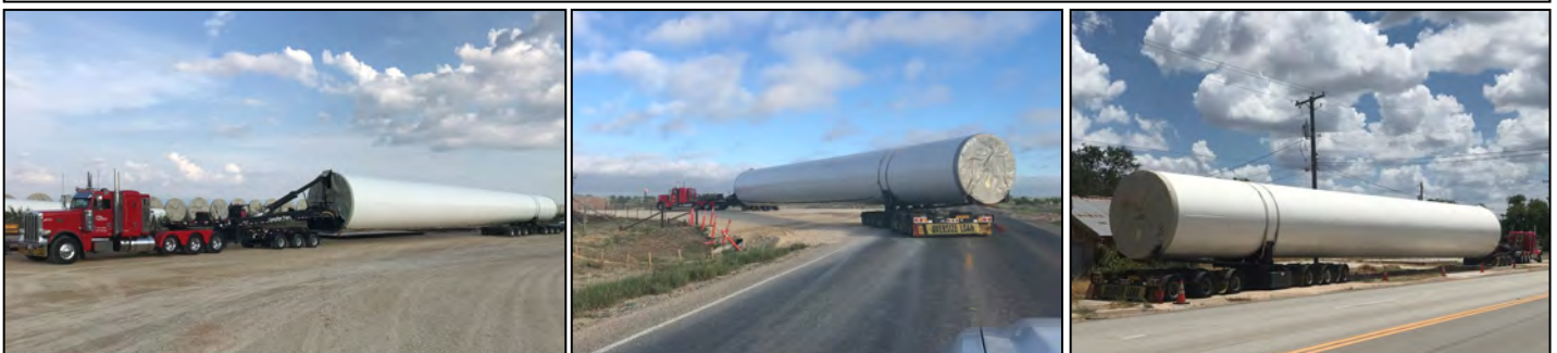
(Above) Brian Johanson (900556) hauling a wind tower section, with dimensions of 189' x 13' x 15'8" and weighing 237,000 lbs. Brian has been with Lone Star since April 1994.
