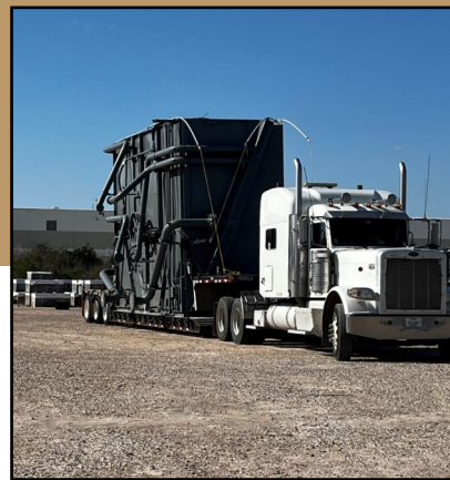
John Heitzman hauling a boiler (featured left) from Alvin, TX to La Porte, TX with loaded dimensions of 110' x 10' 10" x 16' 10" and with a gross weight of 254,000. John has been with Lone Star since March 1999.
