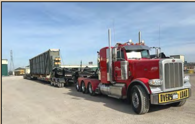
John Heitzman (900558) hauling this convection box with loaded dimensions of 158' L x 10' W x 16' 2" H and weight of 248,000 pounds (featured below)
