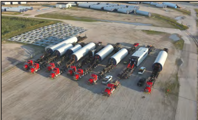
LST Deerfield Wind Project. Photo courtesy of Arturus Espaillat of Atlas Pathfinder, Portland, OR (featured below)
