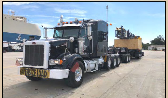
Kenny Brazeal (6446) hauling this drill to Brunswick, GA with loaded dimensions of 118' L x 13' 10" W x 15' 6" H and weight of 172,000 pounds (featured below)
